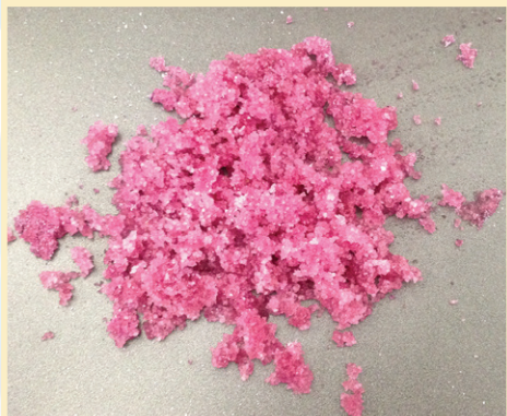
Spilled liquid has been neutralized & absorbed
